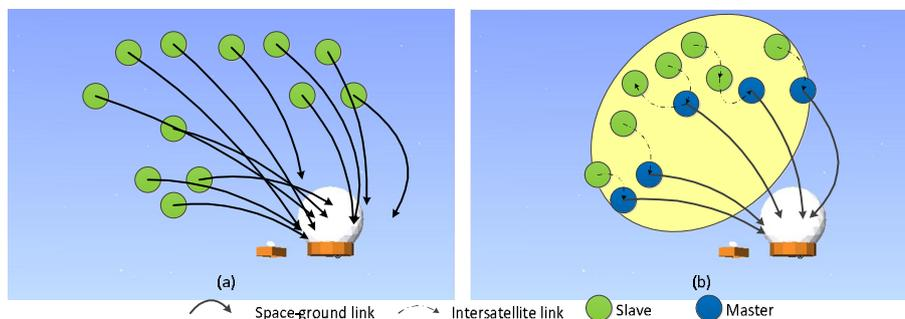
**Figure 1. Multiple Hopping Paths between nanosatellites and ground stations**
