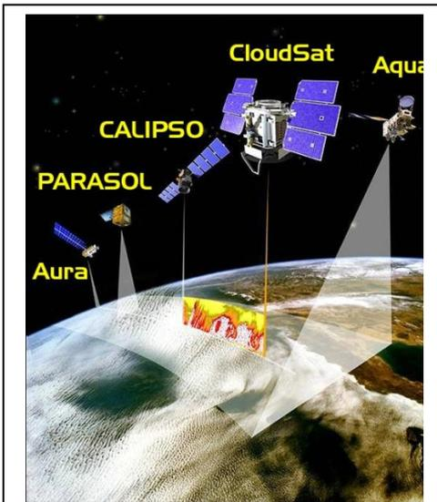
**Figure 1** – This figure shows the A-Train constellation when CloudSat was launched. CloudSat originally flew approximately 12.5 seconds ahead of CALIPSO and, sixty seconds behind Aqua and performed propulsive maneuvers to maintain a 1 km ground track overlap between CloudSat’s and CALIPSO’s
