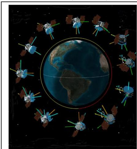
**Figure 5** – This figure shows the vehicle’s orientation over an orbit during the new DO-Op mode. The vehicle collects science data for approximately 54 minutes, hibernates during eclipse, and has brief recovery and setup periods just after eclipse exit and just before eclipse entry.
