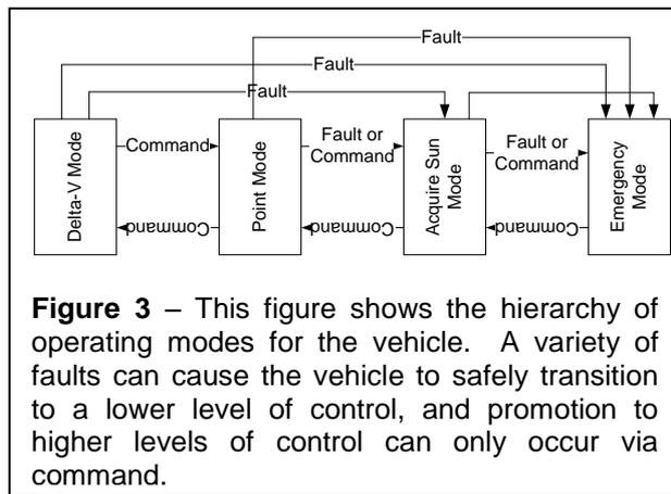
**Figure 3** – This figure shows the hierarchy of operating modes for the vehicle. A variety of faults can cause the vehicle to safely transition to a lower level of control, and promotion to higher levels of control can only occur via command.
