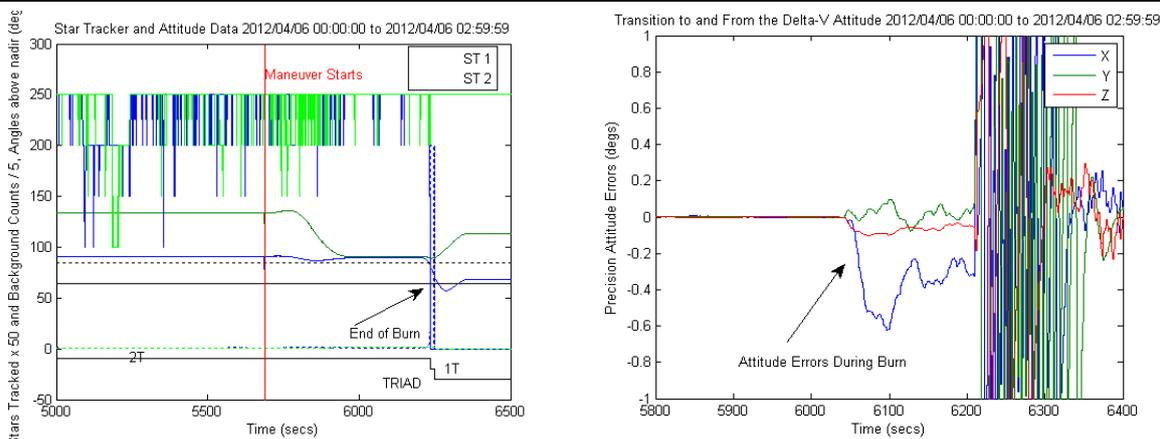
**Figure 11** – Sample performance plots from the 1<sup>st</sup> orbit lowering burn to rejoin the A-Train. During this burn, CloudSat maintained a two star tracker solution through the burn, and the measured attitude errors about each axis were less than 0.7 degrees during the burn. As is shown in Table 1, the burn results were highly accurate, and the delta-V error was 0.14%.
