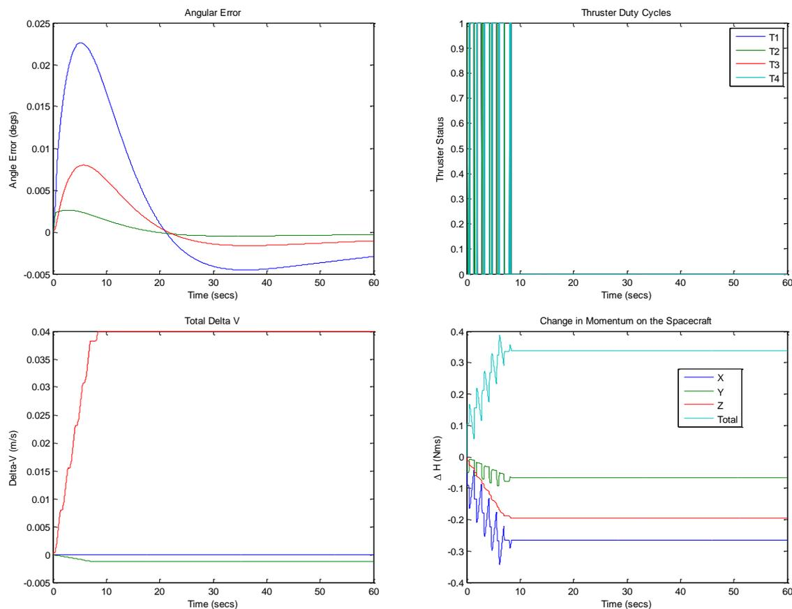
**Figure 8** – This set of figures show the predicted angular deviations during a burn, the thruster duty cycles, the predicted delta-V that is applied to the vehicle and the expected change in the vehicle's momentum state.
