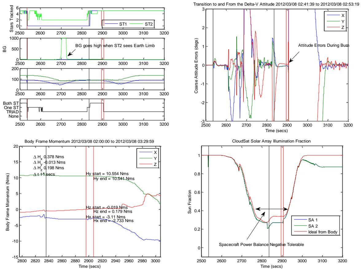
**Figure 12** – This set of figures show that the methodology for performing open loop burns could operate within the spacecraft’s limitations and also still achieve high accuracy results.
