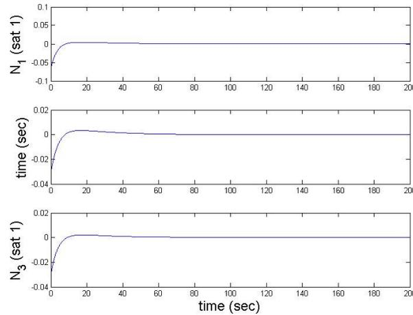
**Figure 4. Time history of the control torque using the proposed SDRE controller**
