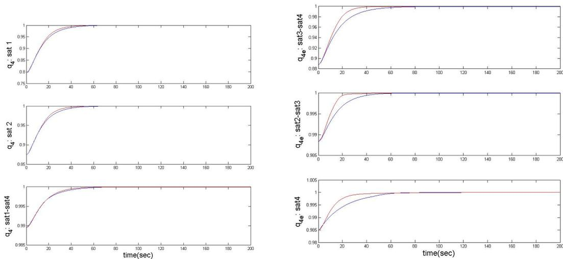
**Figure 3. Absolute and relative attitude histories (formation of 4 satellites) using the proposed SDRE approach (red) and the PD type feedback (blue) of reference [1]**
