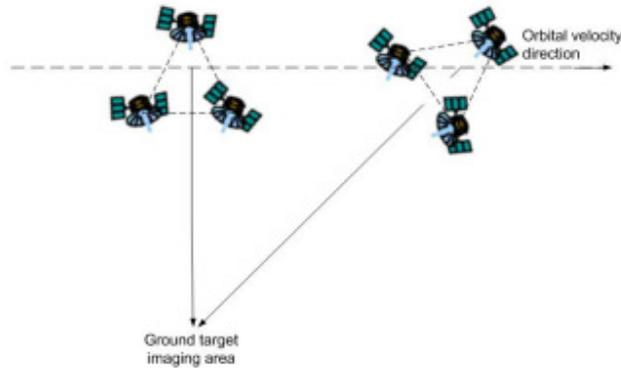
**Figure 1: Example of a synchronised relative attitude scenario**
